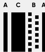
A upholstery B acoustic fleece C insulating core
